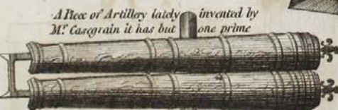
which shoots off both Guns at once There is a ball in each Gun which is chain'd by two bars of Iron that are joined by hinges
